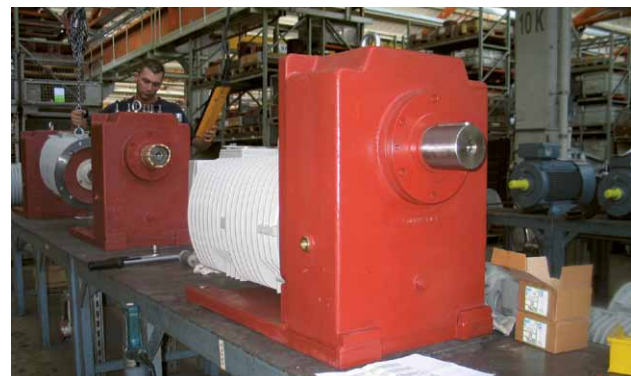
Roller table version, SG200 ARG 200L 8, M_{max}= 1655 \text{ Nm}
