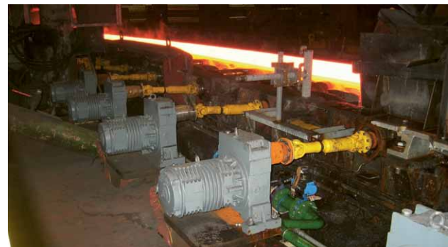
Delay table with S141-1A ARG 160L 4, M_{max}=1039 \text{ Nm}
