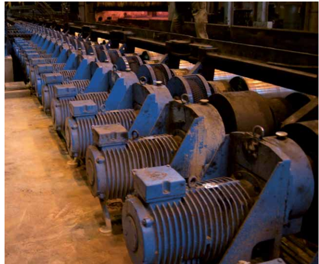
Furnace table with ARG 200L 12, M_{max}=1888 \text{ Nm}
