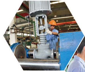
测试阀门内漏及外漏试验 Test the valve leakage and leakage test
